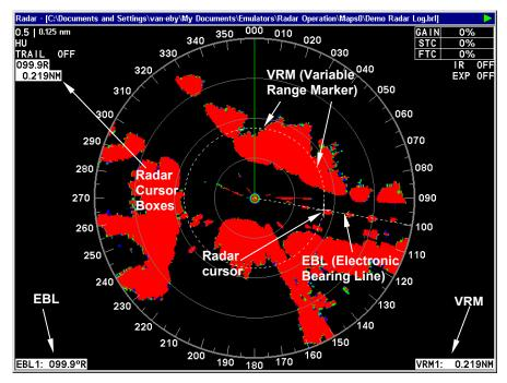
The Variable Range (VRM) shows the target is 0.219 nautical miles away. The Electronic Bearing Line (EBL) displays the target's bearing as 099.9°R.
